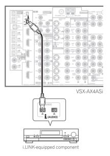
• The arrow on the cable connector body should be lined up with the arrow (to the left of the connector) on the receiver for correct alignment. The i.LINK cable should be inserted straight into the connector so that it snaps easily into place. If not connected properly the receiver will not be able to recognize any connected components. Note that the i.LINK cable is fragile and can be broken easily if too much force is used when connecting.
